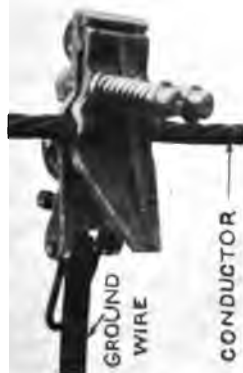
Fig. 8. Grounding Clamp used in Fig. 7, — applied and removed with a switch stick.
